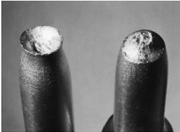
Cup-and-cone fracture in aluminum.
