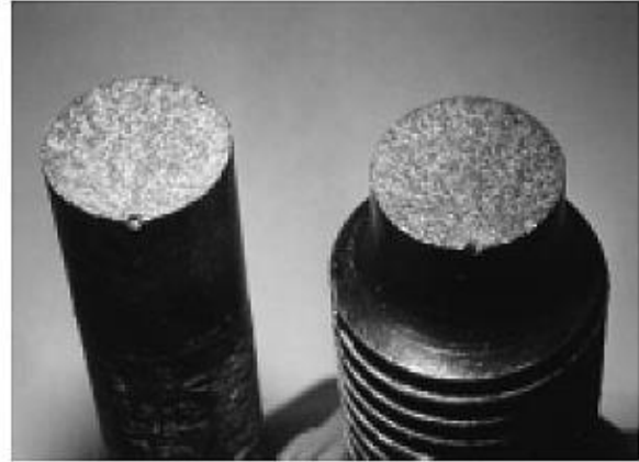
Brittle fracture in a mild steel.
