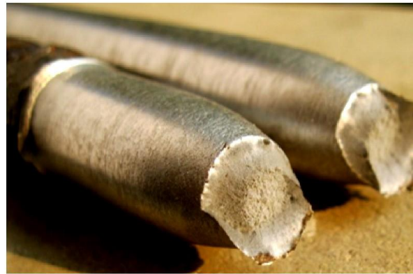
Incomplete Cup-cone fracture (necking found, i.e. Ductile)
