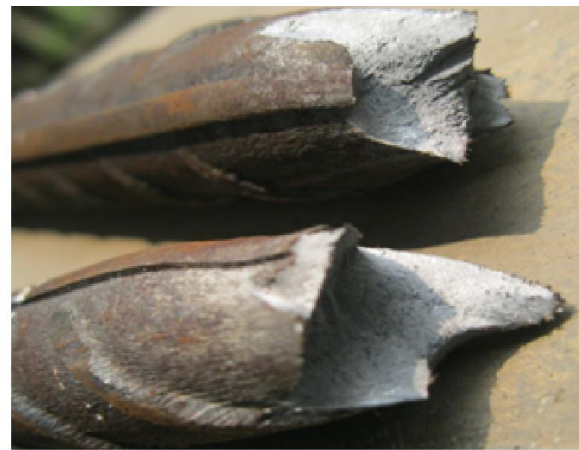
Incomplete Cup-cone fracture (necking found, i.e. Ductile)
