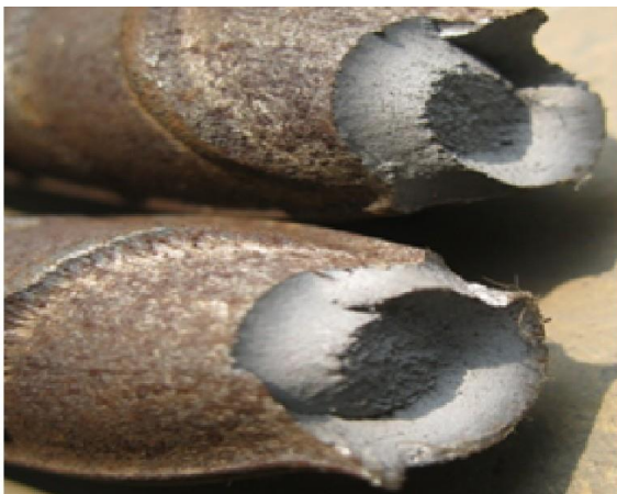
Incomplete Cup-cone fracture (necking found, i.e. Ductile)
