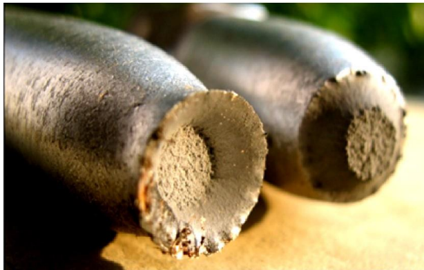
Cup-cone fracture (necking found, i.e. Ductile)
