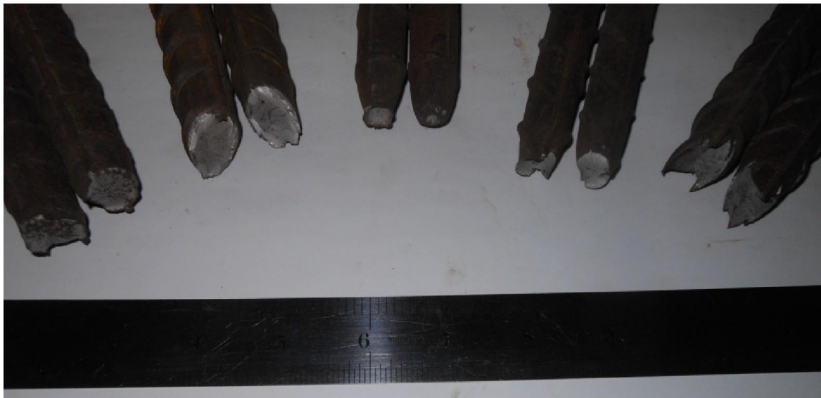
Incomplete Cup-cone fracture (necking found, i.e. Ductile)
